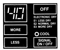
When a number appears in the display and the "cool" light is off, the dryer is counting down a time dry program.
